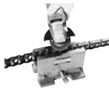
Figure 3: Grinding Down Pin Ends
